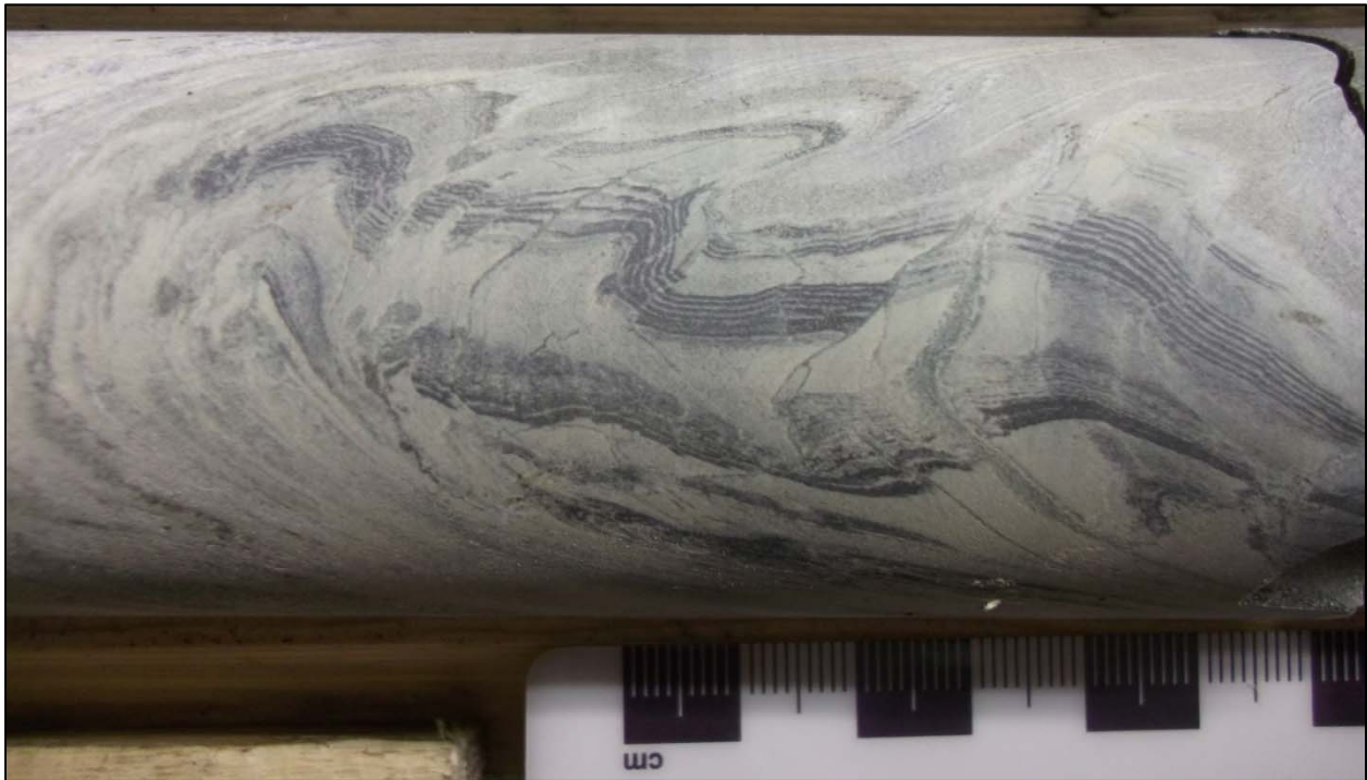
Figure 10-2. Soft sediment deformation in argillite in drill core.
