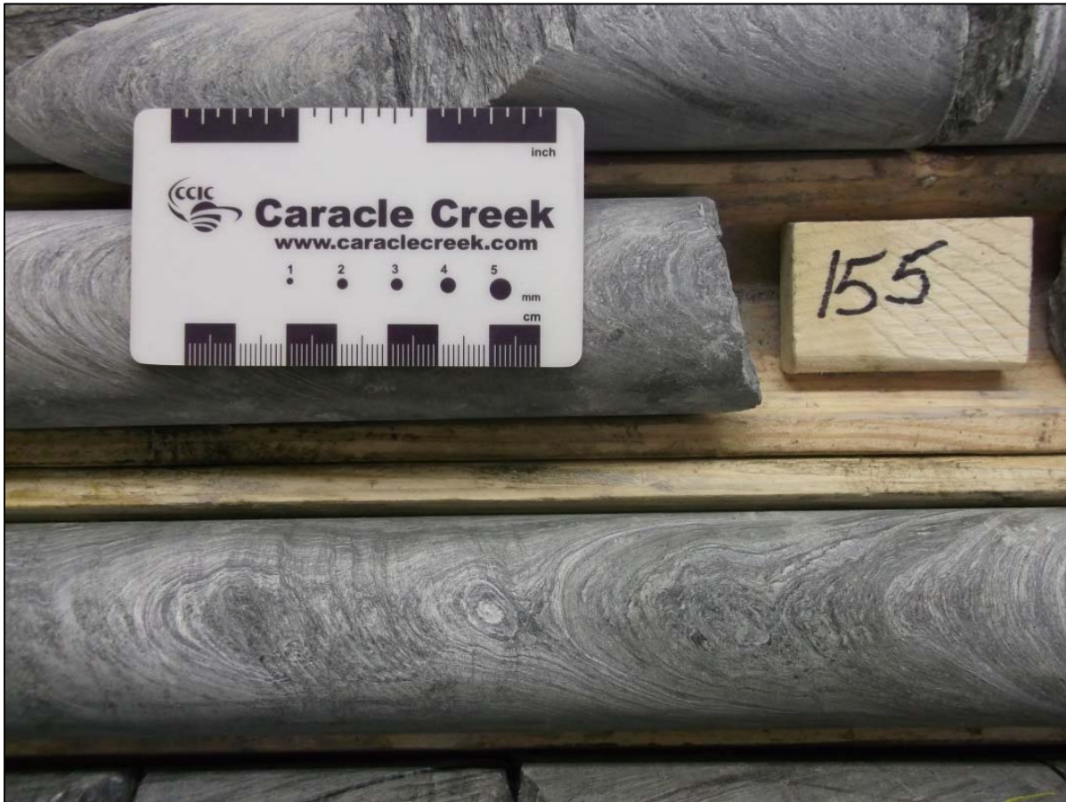
Figure 10-9. Isoclinal folding in core from drill hole AL-13-03.
