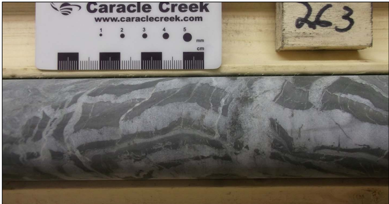
Figure 10-8. Two generations of quartz veins in core from drill hole AL-13-05.
