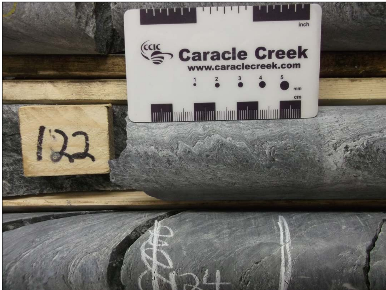
Figure 10-10. Minor folds in core from drill hole AL-13-03.
