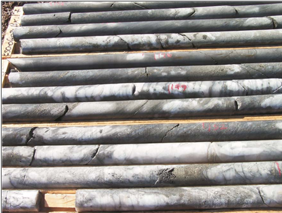
Figure 7-5. Quartz-carbonate veining and vuggy pyrite mineralization in core from drill hole ESO-06-03.
