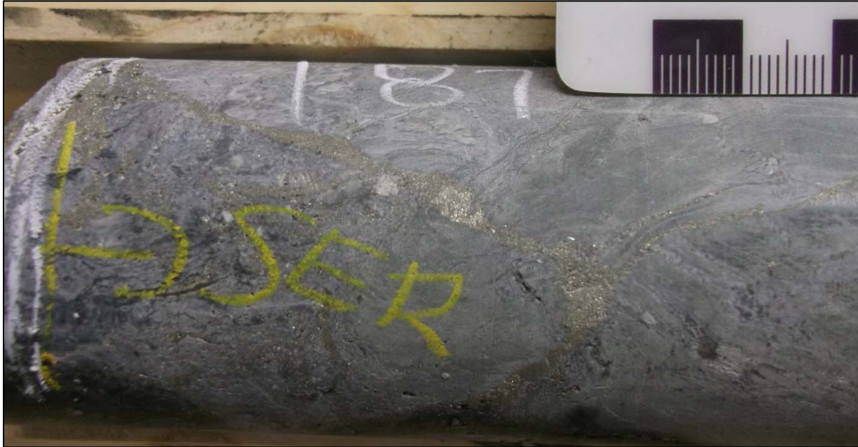
Figure 10-5. Fracture controlled pyrite in core from drill hole AL-13-03.
