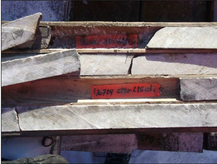
Figure 12-4. Drill core from ESO-06-15, sample 30724 (284 to 285 m), quartz vein.
