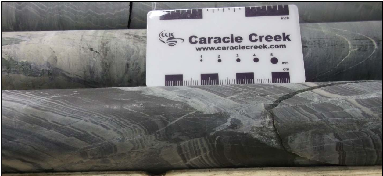
Figure 10-4. Banded iron formation cut by micro-faults in core from drill hole AL-13-05.
