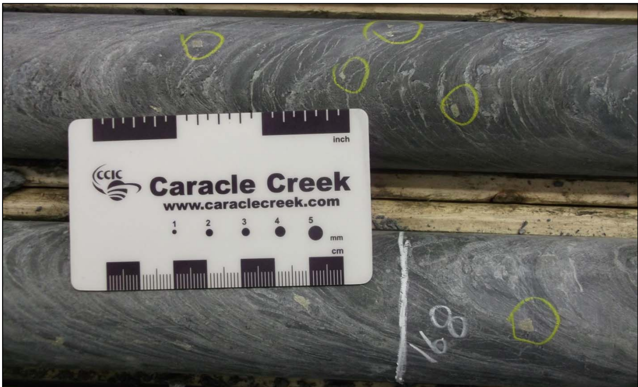
Figure 10-6. Disseminated pyrite in core from drill hole AL-13-03.
