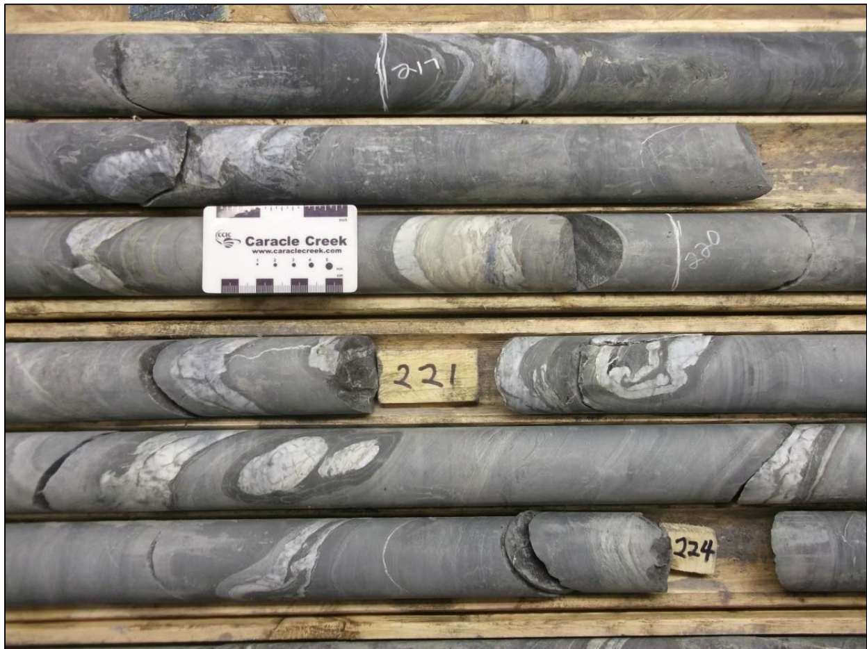
Figure 10-7. Folded quartz veins and pods in core from drill hole AL-13-04.
