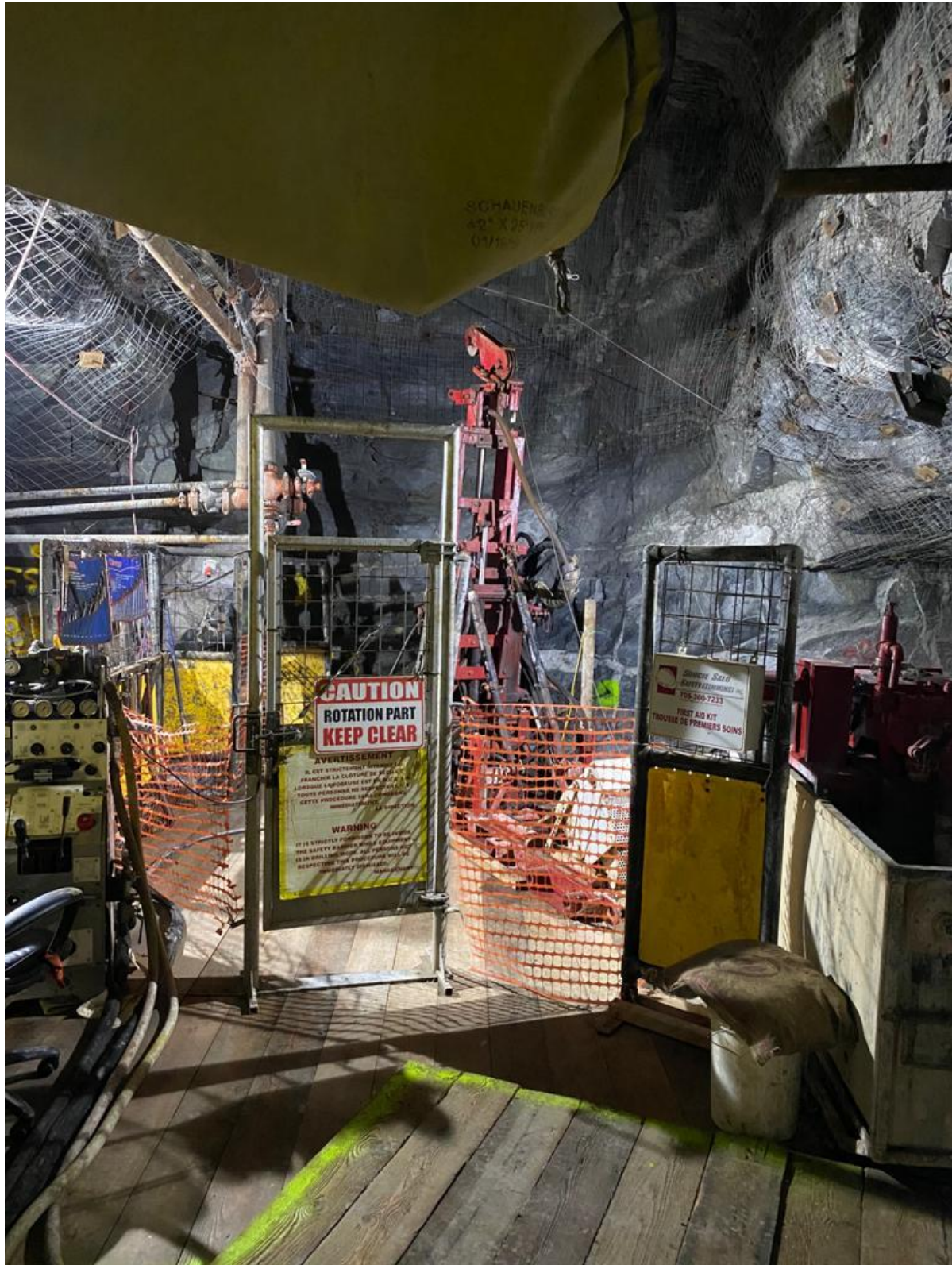
Figure 3: A closer look at the underground diamond drill setup at the second drill pad at the Aureus East project taken by Aurelius Minerals
