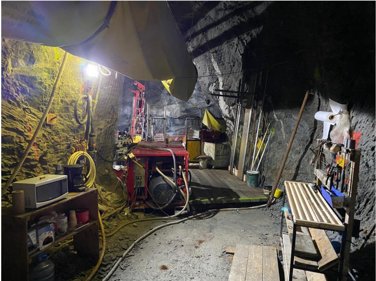
Figure 2: A look at the underground diamond drill setup at the second drill pad at the Aureus East project taken by Aurelius Minerals
