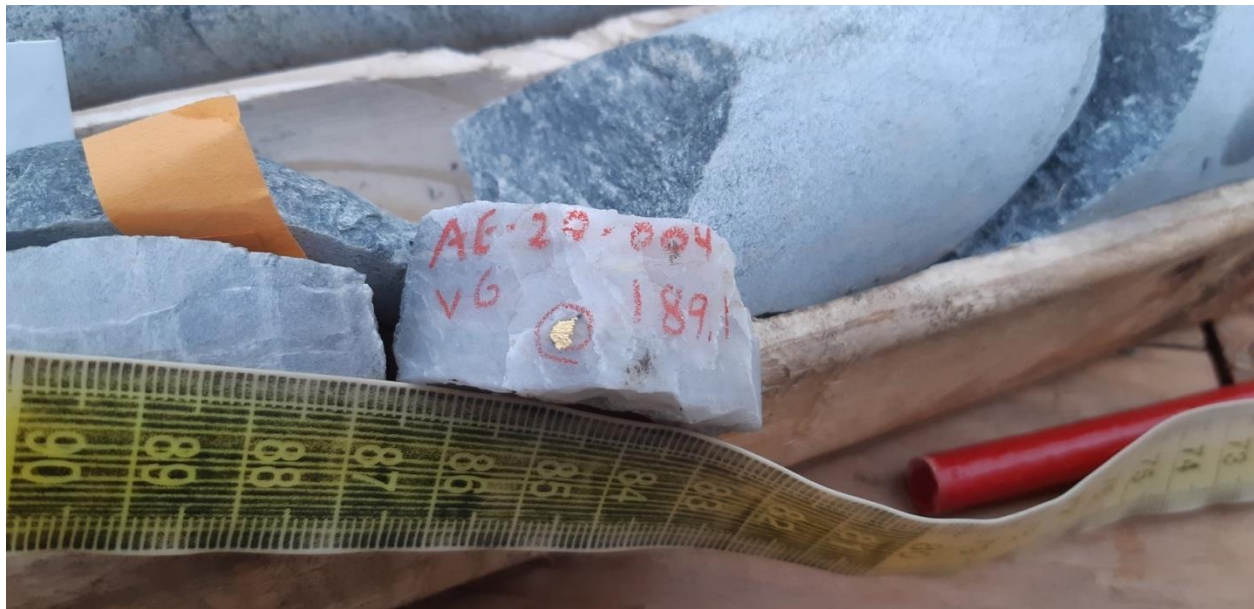
Figure 1: A representative example of core showing visible gold in Hole AE-20-004 at 189.1m, which intersected 0.5m @ 255 g/t gold
