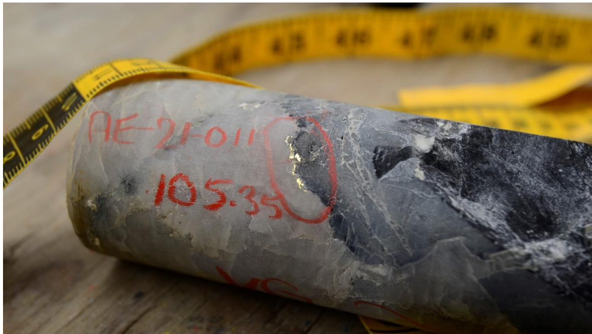
Figure 3: VG Photo 1 Core photo showing visible gold nuggets in hole AE-21-011 at depth of 105.35m.
