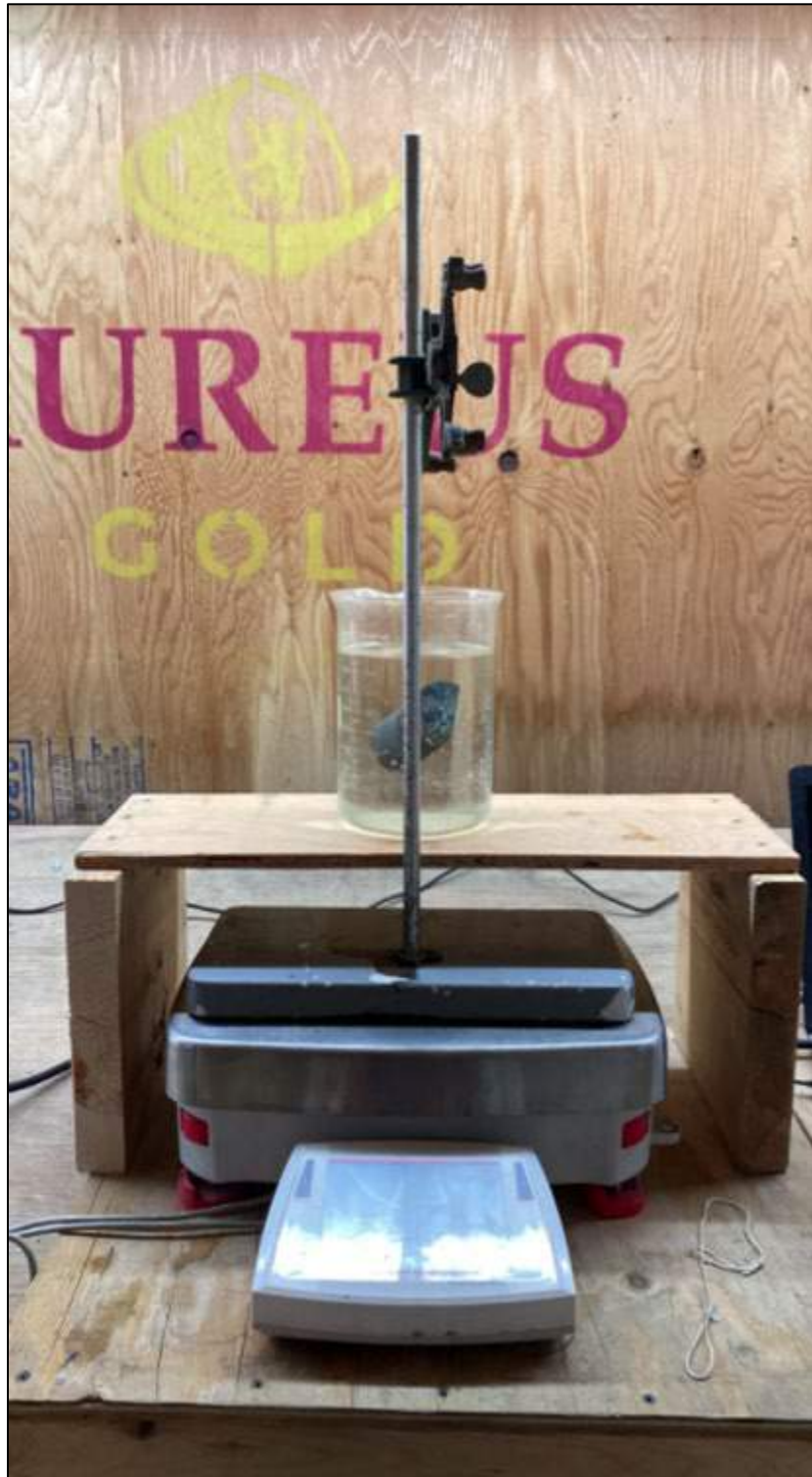
Figure 10-6: Wet SG measurement being recorded
