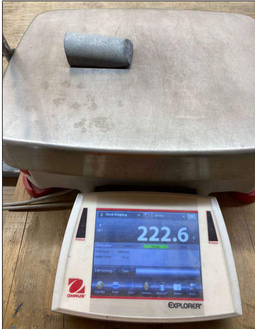
Figure 10-5: Dry SG measurement being recorded
