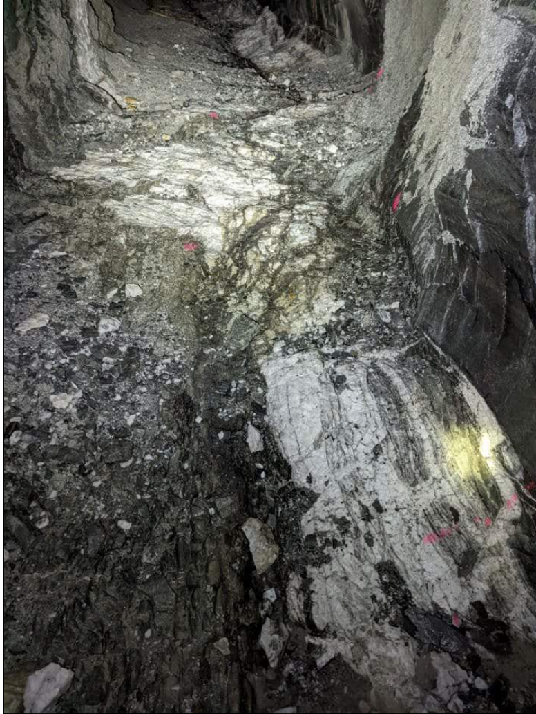
Figure 12-6: Opened mineralized fold limb with mineralized quartz-carbonate veining, argillite, and associated alteration below the 920 level
