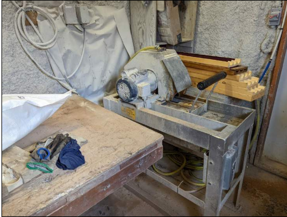
Figure 12-3: Vancon core cutting saw in the core cutting building
