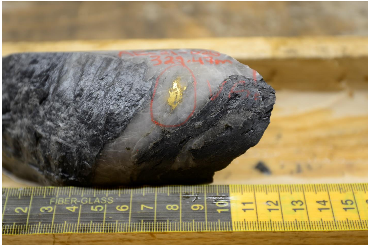
Figure 1: Core photo showing large gold nugget in hole AE-21-026 at a depth of 329.5m – 0.7m sample graded 149 g/t gold
