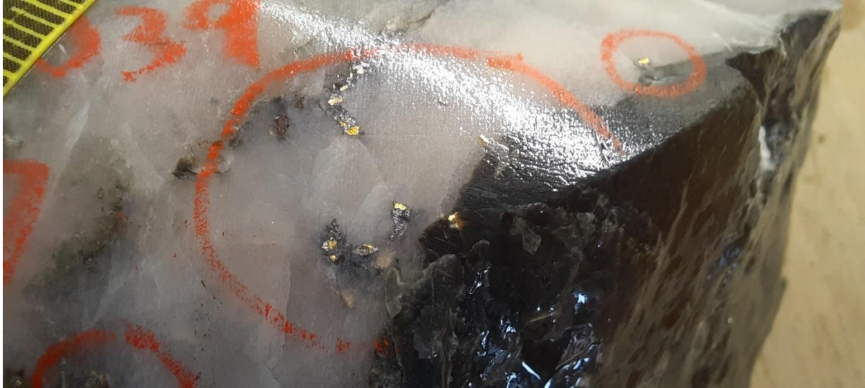
Figure 2: A closer look at the visible gold from Hole AE-21-039 in Figure 1.
