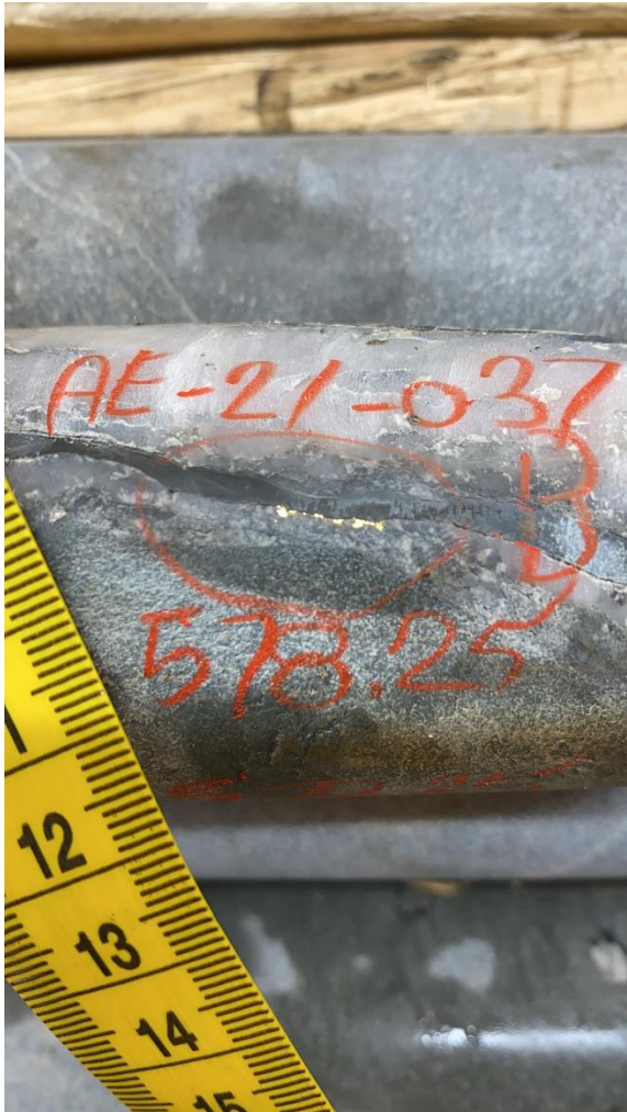
Figure 1: Core photo showing visible gold along the quartz/argillite contact in hole AE-21-037 at a depth of 578.25m – 0.6m sample graded 21.8 g/t gold
