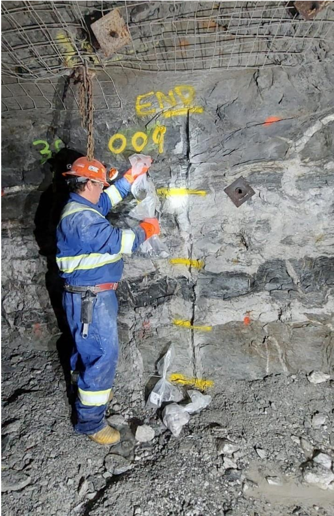
Figure 5: Geo-technician conducting channel sampling of the visible limbs in the floor and walls of the drift at the 940 Level, underground at the Aureus East Gold Project.
